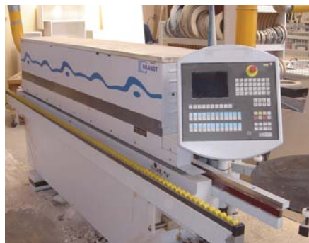
A Morbidelli router and Brandt edgebander form the engine room of the Cooper Webley manufacturing set up.
